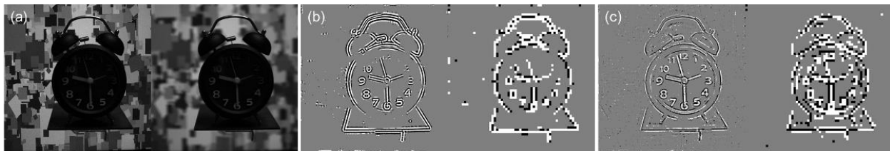
Fig. 2. Light-field background de-cluttering. (a) Sub-aperture image (left) and confocal image (right) from the integration of shifted sub-aperture images. Background de-cluttering in confocal image using bipolar edge filtering: (b) conventional global thresholding loses low contrast details of the OI (e.g., numbers and clock legs) or leave high contrast background clutter while (c) local thresholding of contrast reduction based on MTF of light-field camera keeps all low contrast details of the OI ( 1024\times 1024 in left and 64\times 64 in right). Details of the OI are the more important cues for the object recognition in the low resolution of visual prostheses as shown in right images in (b) and (c).
